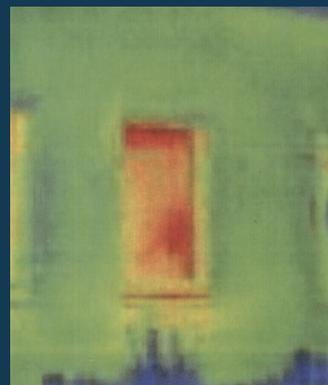
Alt-Isolierglas 3,0 W/m<sup>2</sup>K
